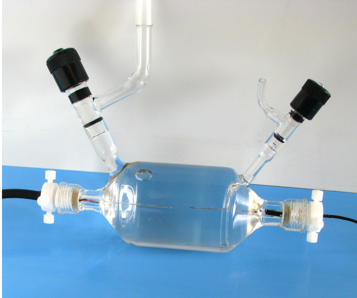
Figure 2.2 – A cylindrical High Purity Cell containing two thermistor probes. Its main function is to keep contaminants away from the point of measurement. The vessel is made out of borosilicate glass and filled with purified water. Each temperature probe contains a small NTC thermistor at the very tip (figure 2.6). Before use, the entire assembly must be cleaned thoroughly and the water must be deaerated.
